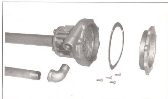
F. Cover, gasket and discharge pipe removed.
