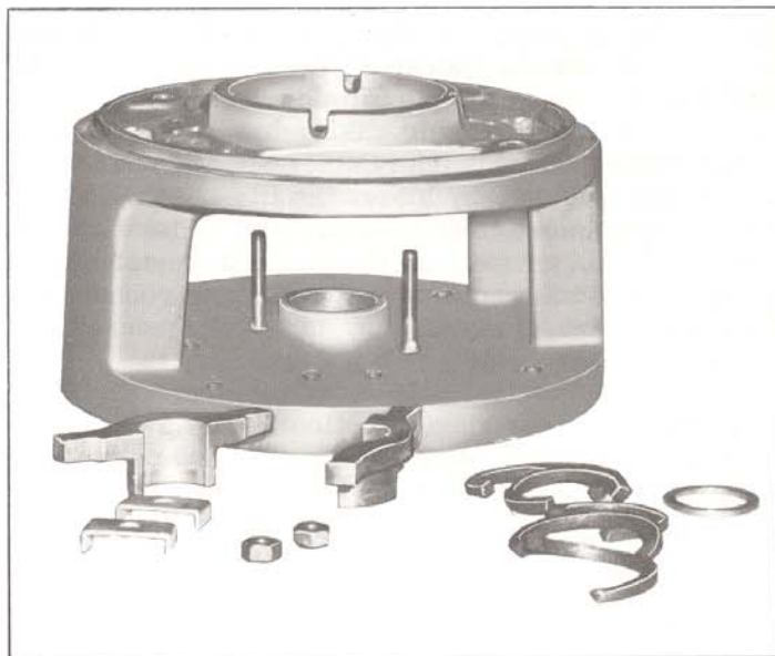
D. Nuts, clamps, gland halves, packing and packing ring removed from lower head.
