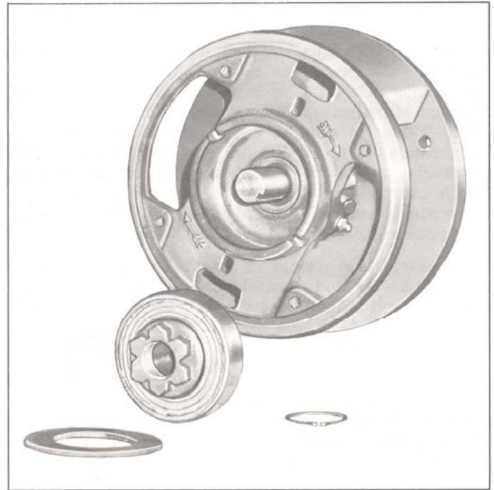
C. Slinger, bearing collar, bearing and retaining ring removed.
