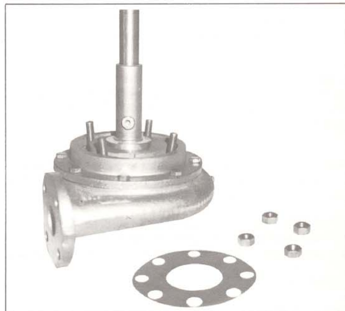
F. Nuts, support piping and gasket removed from cover.
